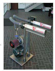
A competitive 20 HP blower can supply 1000 CFM to a 4-air knife drying station at a manifold pressure of 54" WC. At this flow and pressure the maximum exit velocity from an air knife is 29,604 FPM. The exit velocity is an indicator of the air curtain's shear force available for removal of water.
