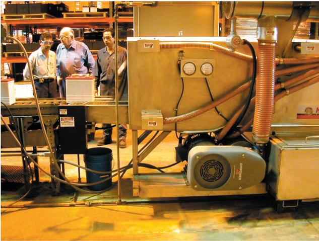
The batteries then proceed through a drying section featuring Vortron air knives, also Type 316 SS, supplied with heated air from a Vortron **AirPower™** Z40 blower. The high-performance **AirPower™** Z40 blower develops 100 in-Wc at 1,000 SCFM (and 75% efficiency!) to supply an array of five air knives. This extraordinary performance from the single Z40 blower produces an amazingly high air-knife exit velocity, sufficient to flash dry surfaces at considerable distances.
