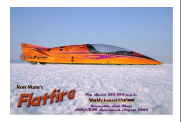
The FlatFire is powered by a Vortech V-1 T-Trim supercharged flathead Ford V8.
