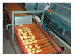
The Australian Potato Industry conducted several trials to determine whether or not air drying would be effective in minimizing the soft rot commonly found in "tubers" (potatoes). One recommendation was the application of air knives to dry the potatoes. Air-knife drying is an alternative that overcomes many of the problems of the sponge roller.
