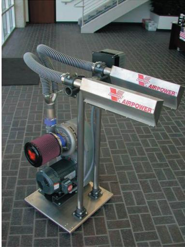
A competitive 20 HP blower can supply 1000 CFM to a 4-air knife drying station at a manifold pressure of 54” WC. At this flow and pressure the maximum exit velocity from an air knife is 29,604 FPM. The exit velocity is an indicator of the air curtain’s shear force available for removal of water.
