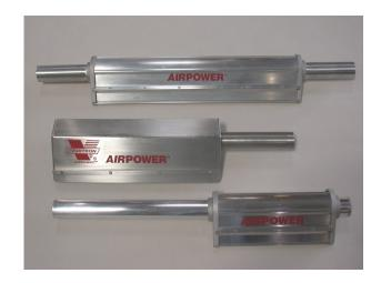
Vortron's **AirPower**<sup>™</sup> line of air knives can be supplied either in extruded aluminum or stainless steel. We manufacture air knives with manifold sizes of 3.5" and 5" and lengths up to 154 inches. Since our air knife gap (slot size) is adjustable we can supply a range of gaps from 0.015" up to 0.070". This flexibility in air knife gap allows us to design the airflow (volume) to match the application needs.
