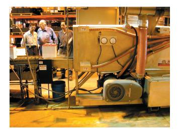
The batteries then proceed through a drying section featuring Vortron air knives, also Type 316 SS, supplied with heated air from a Vortron *AirPower<sup>TM</sup>* Z40 blower. The high-performance *AirPower<sup>TM</sup>* Z40 blower develops 100 in-Wc at 1,000 SCFM (and 75% efficiency!) to supply an array of five air knives. This extraordinary performance from the single Z40 blower produces an amazingly high air-knife exit velocity, sufficient to flash dry surfaces at considerable distances.
